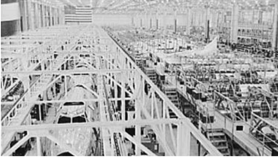
Figure 35. A B-17 bomber under construction at a Douglas Aircraft factory at Long Beach, California. Image courtesy of Library of Congress.
