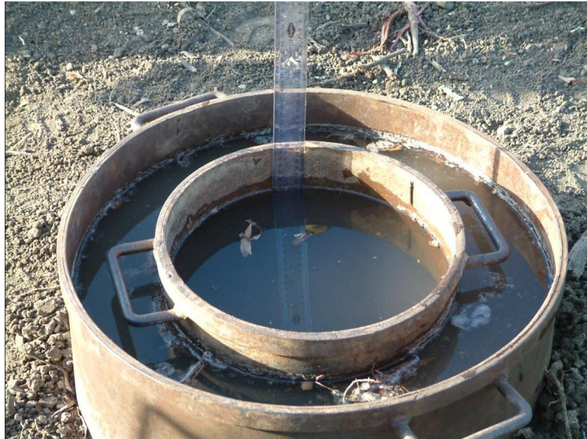
Figure VII.5. Photo of Simple Double Ring Infiltrometer
