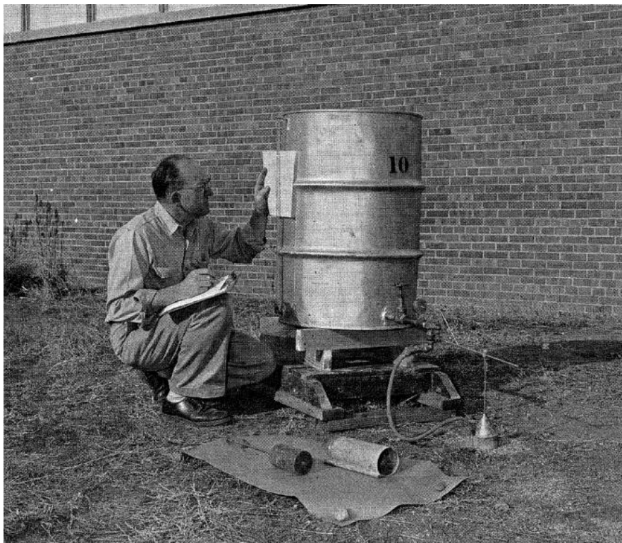
Figure VII.13. Typical Well Permeameter Test Installation
