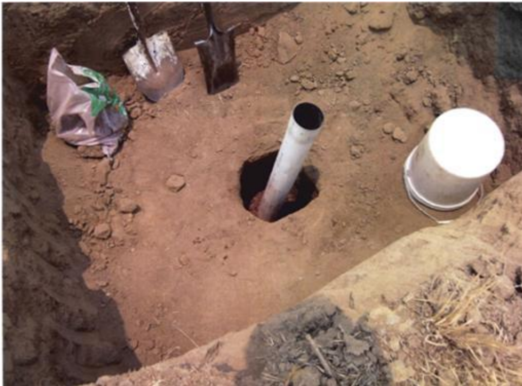
Figure VII.17. Photo of Percolation Test Pit.
