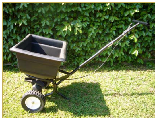
Fertilizer spreader. Make sure to set the spreader to the proper application rate to avoid excess fertilization.
