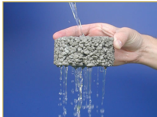
This is a demonstration of porous concrete. Most of the water is able to percolate through. Courtesy of The Southeast Cement Association
