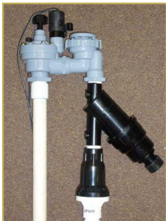
Drip valve with a filter and pressure regulator. This picture shows an anti-siphon valve followed by a filter and a pressure regulator.
